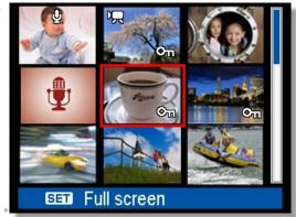
Use the four-way control to select the desired image, and press [T] or the SET button to show the selected image in full screen.
