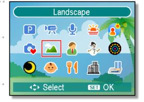
Use the four-way control to select a desired mode and press the SET button to confirm the setting.
